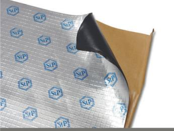
**STP BOMB** – self-adhesive bituminous-mastic vibration damping material. It is a three layer combination that consists of a bituminous layer and an adhesive mounting layer on the mastic base covered by an antiadhesion paper. The facial covering is an aluminum foil.
