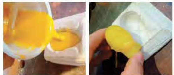
Figure 31.4: Pour pigmented resin in mold and remove finished workpiece when cured.
