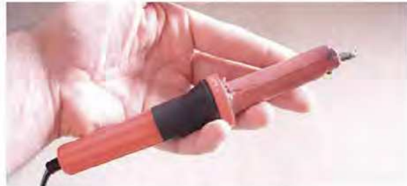
Figure 32.2: Silicone protector on the soldering iron.
