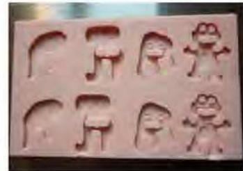
Figure 35.13: Milled candy molds.
