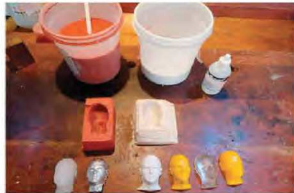
Figure 30.6: High-temperature molding (left) and low-temperature molding (right).
