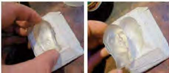
Figure 31.5: Adding talcum powder to resin mixture.
