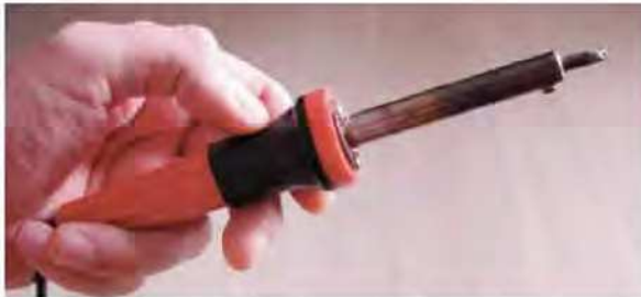
Figure 32.1: The long metal part of a soldering iron invites burns.
