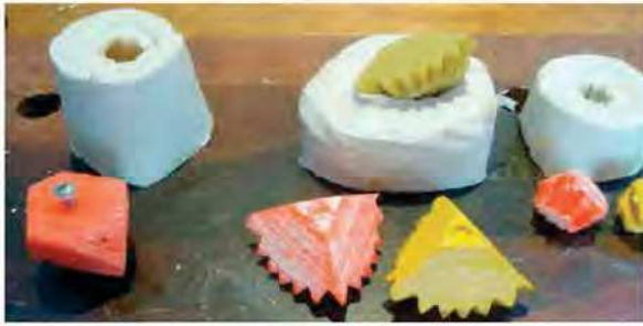
Figure 31.7: The red workpieces were 3D printed. The yellow ones are copies made from a mold.
