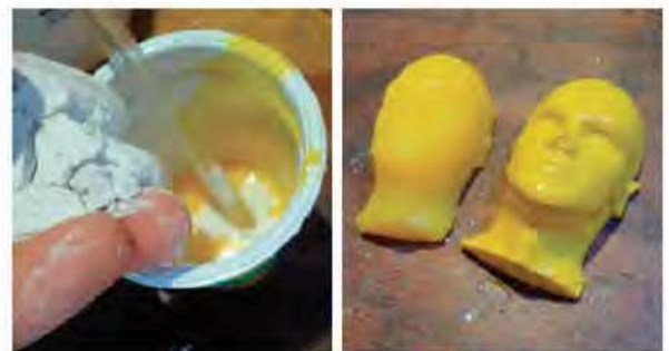
Figure 31.5: Adding talcum powder to resin mixture.
