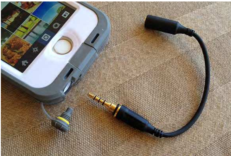
LifeProof headphone adapter connector detail
