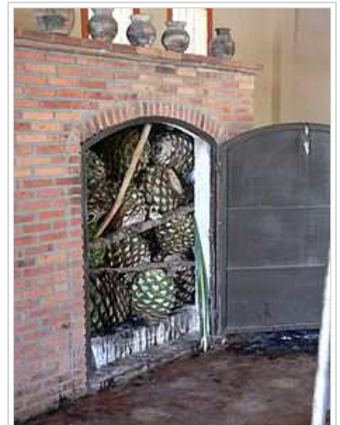
A distillery oven loaded with agave piñas or "pineapples", the first step in the production of tequila post harvest.
