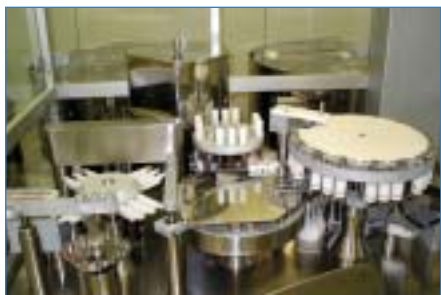
Figure 7: Equipment for integrated filling and assembly of DirectHaler Nasal.
