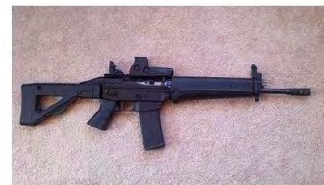
A SIG556 Classic equipped with an EOTech 512 holographic weapon sight and STANAG magazine.
