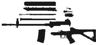
SG 550 disassembled into its main constituent groups
