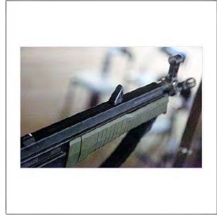
Detail of the top-mounted arming lever of the C42
