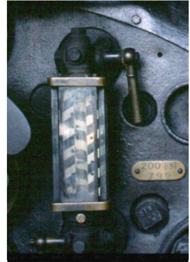
Water gauge on a steam locomotive. Here the water is at the "top nut", the maximum working level. Note the patterned backplate to help reading and toughened glass shroud .
