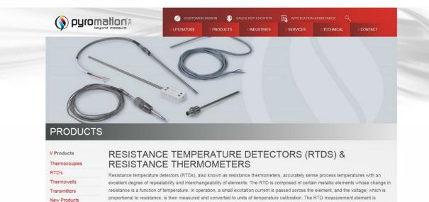
resistance is a function of temperature. In operation, a small excitation current is passed across the element, and the voltage, which is proportional to resistance, is then measured and converted to units of temperature calibration. The RTD measurement element is manufactured by winding a wire (wire wound elements) or plating a film (thin film elements) on a ceramic or glass core and sealing the element within a ceramic or glass capsule.
