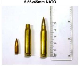
5.56×45mm NATO with measurement, left to right: projectile, empty case, complete round with projectile in case
