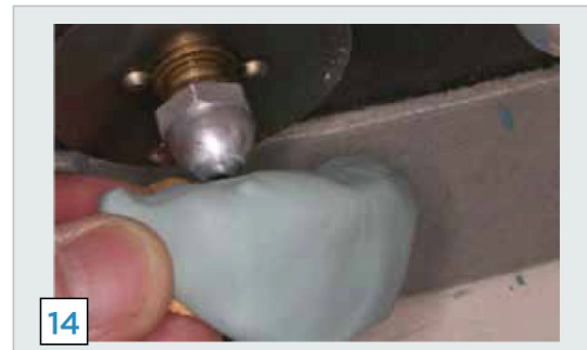
FIG 14. Melted wax being injected through one of the holes.
