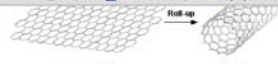
graphene sheet SWNT Copyright Professor Charles H. Lieber Group An excellent description of Carbon Nanotube Tips for Atomic Force Microscopy
