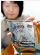
Bridgestone engineers developed this Quasa thegripase Liquid Powder Display, a flexible digital screen, using nanotechnology. Tommaso Tassinari/Prattimedia
