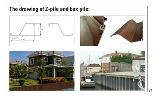
The JD Fields & Company website contains a page captioned "Sheet Piling 101" referencing the "Z" shape of certain sheet piles and stating that "'Z' pile interlocks are located on the outer edges of the section, which not only results in higher module and inertial properties, but the interlock rotation issue does not apply."<sup>28</sup>
