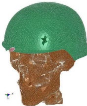
Fig. 3: The complete FE model includes headform, helmet, and bullet.
