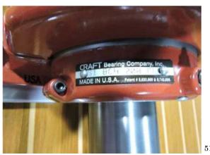
Second, Opposer establishes that it is the only concern that manufactures split bearings in the United States.<sup>52</sup> A "split bearing" is split in half, facilitating installation and repair around cylindrical shafts, as its catalog cover shows:
