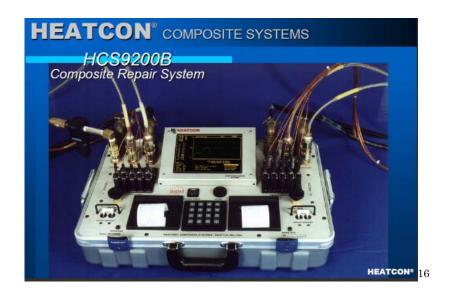
We find the '519 patent discloses the utilitarian advantages of the arrangement of the various parts, e.g., vacuum ports and pumps, power ports, printers and monitor, of an interface for a portable hot bonder. Given the strong weight to be accorded patent evidence under TrafFix, we find that the patent is sufficient to establish  $prima\ facie$  that the design is functional.
