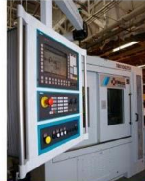
Wera Profiator gear profiler run by a Sinumerik 840D, the highest level CNC in the Siemens line, used for fully automated production of ring gears.
