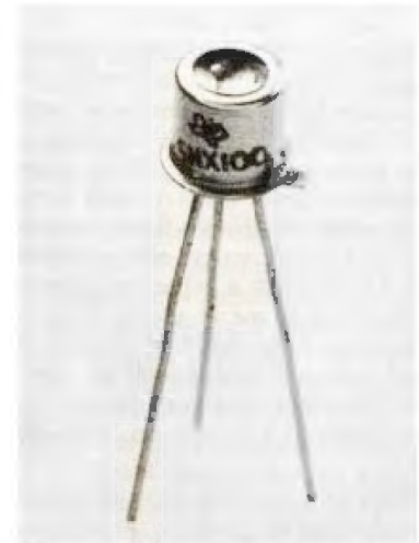
A Texas Instruments SNX-100 GaAs LED contained in a TO-18 transistor metal case.
