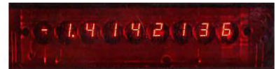
LED display of a TI-30 scientific calculator (ca. 1978), which uses plastic lenses to increase the visible digit size
