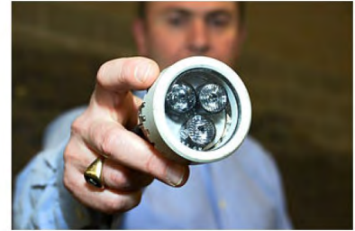
LED for miners, to increase visibility inside mines
