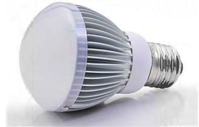
A bulb-shaped modern retrofit LED lamp with aluminium heat sink, a light diffusing dome and E27 screw base, using a built-in power supply working on mains voltage
