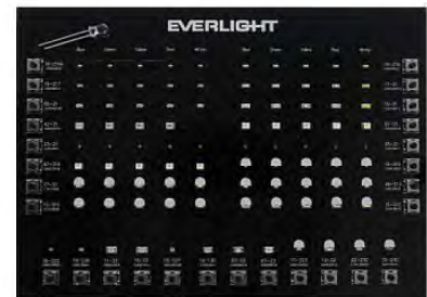
Photo of miniature surface mount LEDs in most common sizes. They can be much smaller than a traditional 5 mm lamp type LED, shown on the upper left corner.
