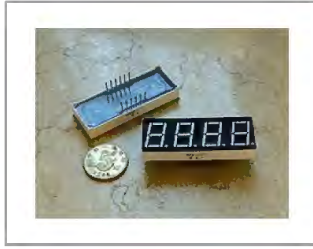
LED digital display that can display four digits and points
