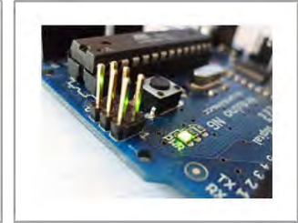
A green surface-mount colored LED mounted on an Arduino circuit board
